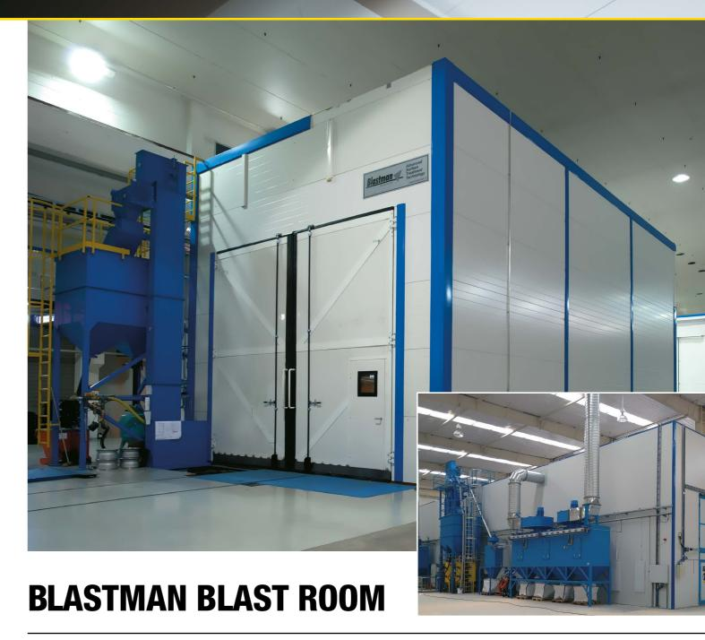
The blast cleaning process must be isolated from the surrounding environment due to the nature of the process. Typically, blasting takes place in a sealed enclosure or room. The design and structure of the room should be strong and well protected against blasting. The room should be well sealed to avoid any leakage of abrasive, dust, and noise. In order to serve our customers with turnkey solutions, we have developed our Blastman blast rooms for different applications.
